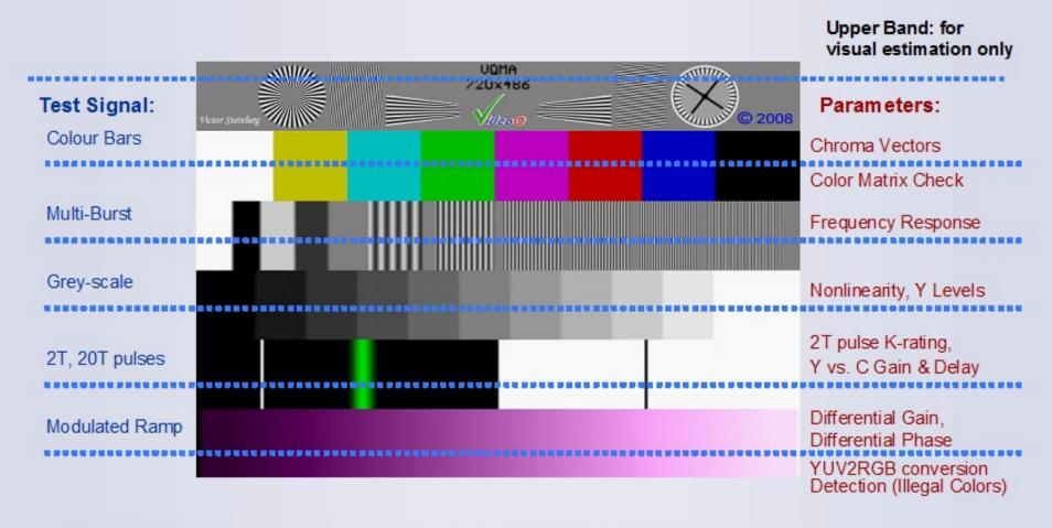
Noise & Interferences accurately measured on any static image by analysis of frame differences
